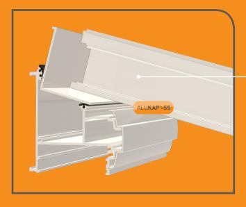
4. Cut the first ALUKAP®-SS High Span/Low Profile base bar to the correct length to allow it to rest between the top and bottom ALUKAP®-SS Bar Caps. Measure the bolt fixing position from the end of the ALUKAP®-SS base bar for drilling a hole through the ALUKAP®-SS Span base bar and down through the bold flange on the ALUKAP®-SS Eaves Beam and Wall Plate. This will vary between 40mm and 70mm depending on the pitch).
